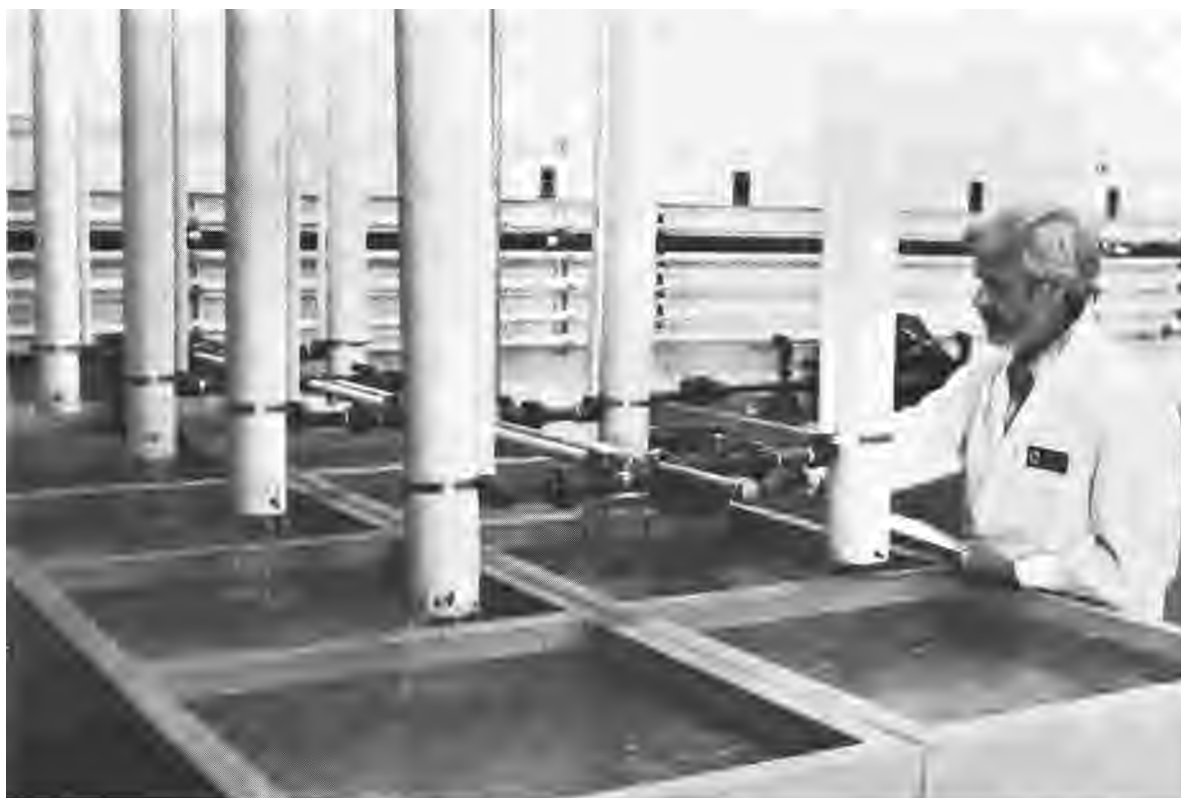
Research requires fish that are free of stresses that may be caused by problems in the water supply. These column aerators developed at the La Crosse National Fishery Research Laboratory are highly efficient for producing nitrogen and oxygen levels that are suitable for fish culture and testing. Photo by T. D. Bills.
