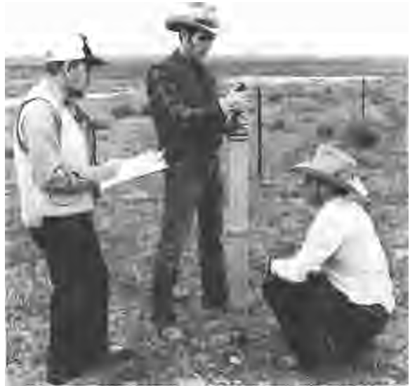
Biologists measure the force required to trigger an M-44 sodium cyanide ejector. The test apparatus protects observers from contact with the ejected NaCN. The desired pull force is 3-4 pounds and units that do not eject at pull forces below 8 pounds are considered to be defective. Photo by G. Connolly.
