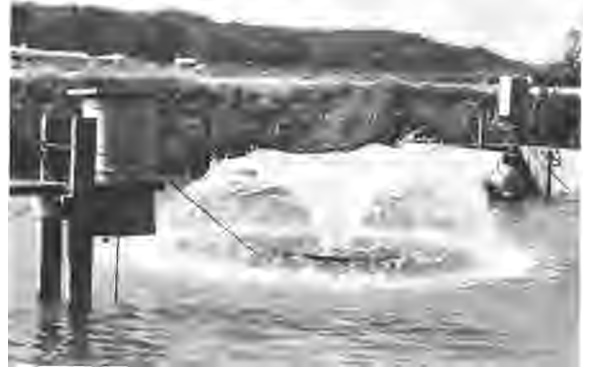
Fountain and spray-type floating agitators are used to provide emergency aeration in warmwater fish ponds. The device mounted above the water at left is a demand feeder, which delivers food when the rod extending from the can to the water is moved by the fish. Photo by M. A. Suttle.
