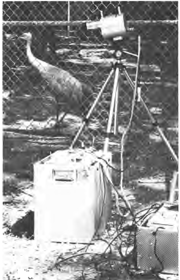
Circular variable filter spectrometer is used to measure spectral reflectance of a sandhill crane. Photo by J. Payne.
