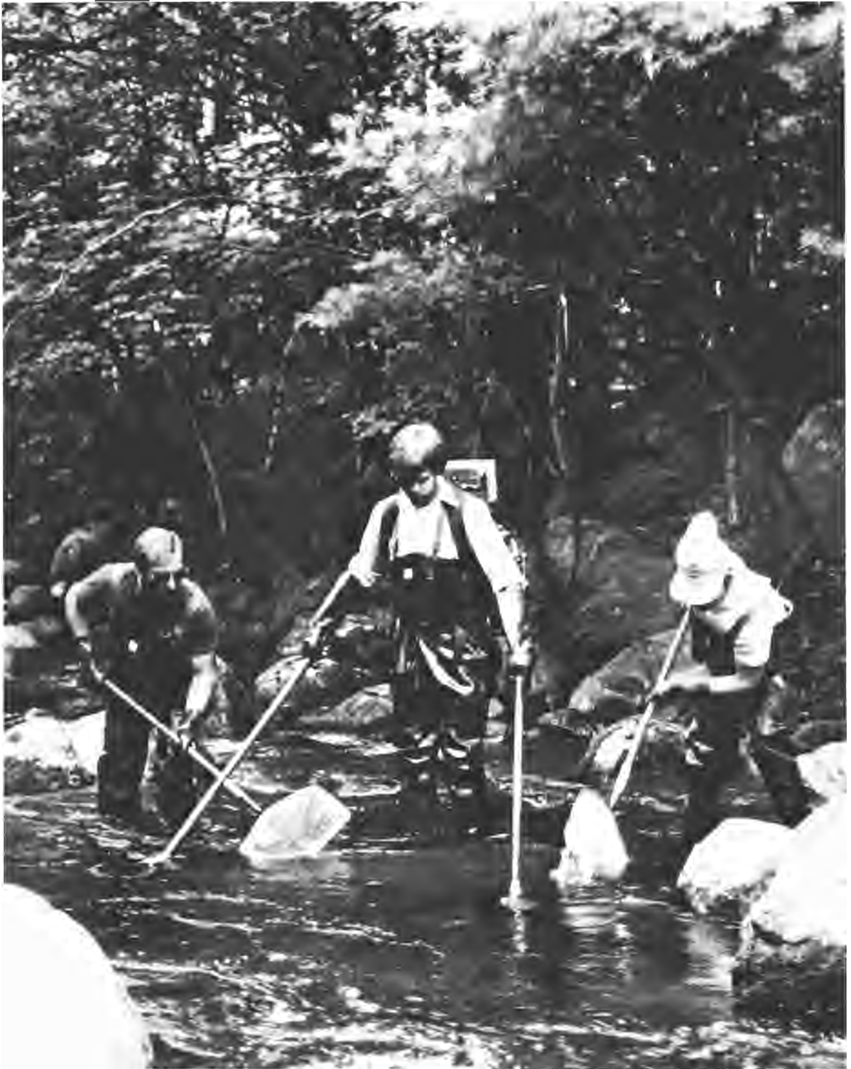
Electrofishing is the most commonly used technique for fish population estimates in streams. In this small Virginia trout stream, one technician maneuvers the electrodes (powered by a back-pack generator) while two others collect stunned fish with dip nets. A fourth (not shown) transfers the fish to a live-box for temporary retention until they are fin-clipped or tagged and released. When the operation is later repeated in the same section of stream, the relation between the number of marked and unmarked fish caught is the basis for the population estimate. Photo by G. B. Pardue.
