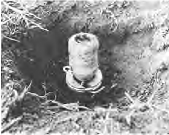
The M-44 sodium cyanide ejector is an important tool for removing coyotes from livestock ranges. About two-thirds of all Animal Damage Control program use of M-44's is in Texas. Because current M-44 ejectors frequently malfunction, research is in progress to improve the performance of this tool. Photo by G. Connolly.
