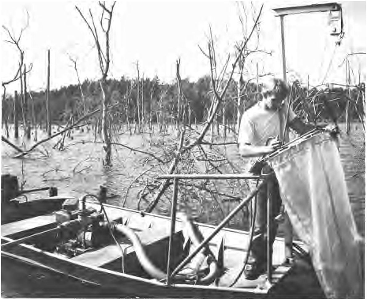
High-volume pump being used to sample larval fishes in standing timber plots in Georgia. The cover provided by such plots may be an important factor in survival of larval fishes. Photo by R. Petering.
