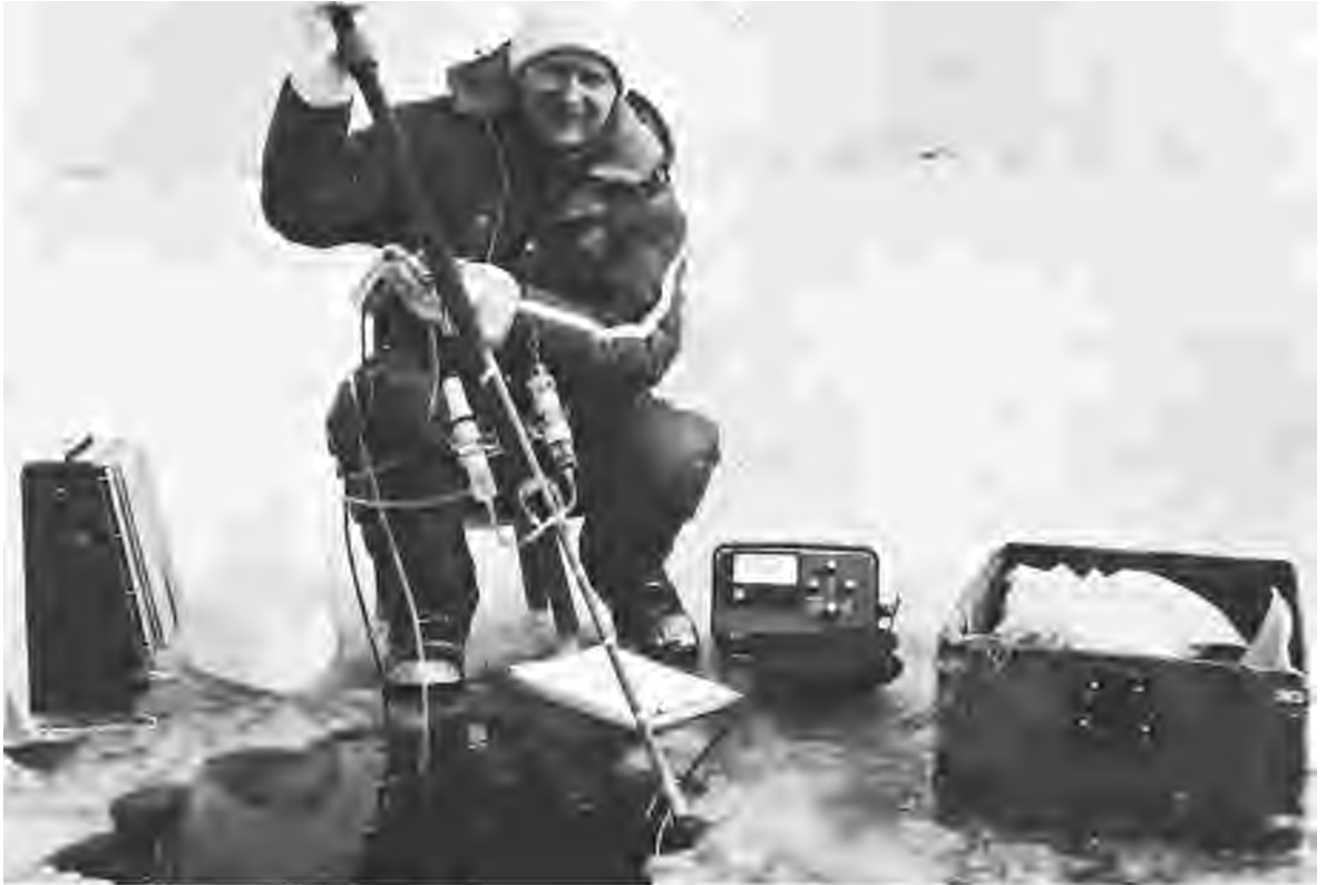
Limnologist preparing to deploy a probe designed to measure dissolved oxygen and hydrogen sulfide under ice, within the interstices of rock-rubble substrate used historically for spawning by lake trout in Lake Huron. The probe has been used successfully to obtain interstitial water quality measurements as deep as 30 cm beneath the surface of the substrate. An underwater television camera (not shown) is used to assist in positioning the probe at the desired level within the substrate. Photo by J. K. Hiltunen.
