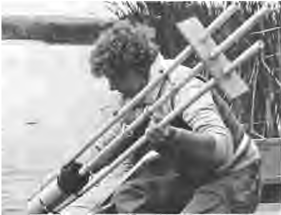
To help evaluate level ditch habitat in the production of aquatic invertebrates, a biological technician collected samples with a benthic core sampler in eastern South Dakota. Photo by M. R. Broschart.
