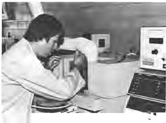
Chemist analyzing wildlife tissue for metal content using an atomic absorption spectrophotometer. The detection of contaminant residues in wildlife tissues contributes to the evaluation of contaminant effects on wildlife and their habitats. Photo by H. Bourne.
