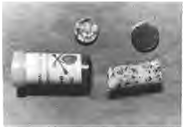
Caking or decomposition of sodium cyanide currently is reducing the effectiveness of M-44's used by the Animal Damage Control program. In this capsule, the powdered NaCN mixture has solidified into a hard mass (right). If ejected into a coyote's mouth, this "pill" would be spit out before the toxicant could take effect. The "educated" coyote would probably never pull another M-44. Because caking or decomposition of NaCN results from moisture inside the capsule, improved sealing of capsules is expected to solve the problem. Photo by G. Connolly.
